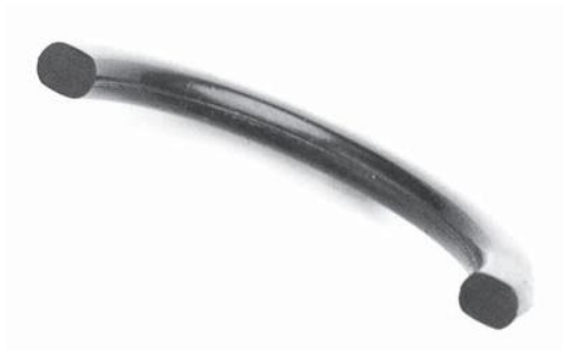
Fig. 9.9 Characteristic compression set. High deformation
