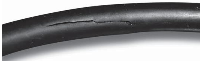
Fig. 9.12 O-ring damaged by explosive decompression
