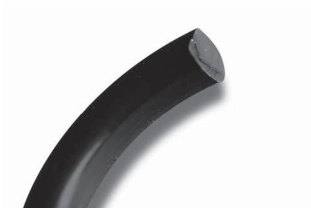
Fig. 913 Wear is seen as flattening of O-ring on one side
