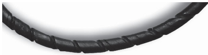
Fig. 9.10 Twisted O-ring with spiral marking
