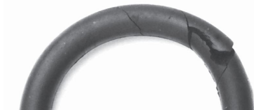
Fig. 9.11 Twisted O-ring with spiral cuts in surface
